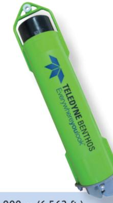
**The R12K Deep Water Acoustic Transponding Release** is designed for full ocean depth mooring recovery applications requiring a highly-reliable rugged stainless steel package and 4,540 kg (10,000 lbs) load handling.
