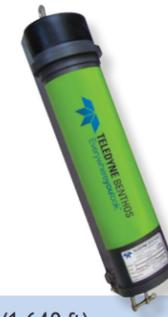
**Model R2K Mid-Water Acoustic Transponding Release** is a full function acoustic release in a rugged and compact stainless steel housing for use in depths to 2,000 meters and loads up to 2,000 kg (4,400 lbs).
